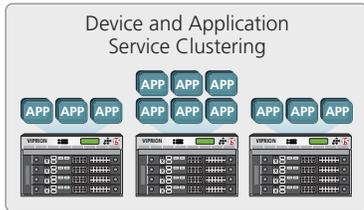
Device and Application Service Clustering provides true scale out of BIG-IP devices, automatic configuration syncing, and failover of specific application workloads in an active N+1 device cluster.
